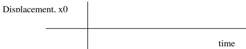
Logarithmic decay ( rate of decay )  $\delta = 1/N \ln (X_0 / X_n)$ . High  $\delta$  values indicate high damping ie higher loss of energy.
